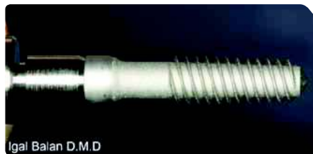
Fig.3 Cortical implant (4X18 mm) with an aggressive thread for a better primary stability and with a smooth neck surface for reduction of bacterial adherence and inflammatory process development.
